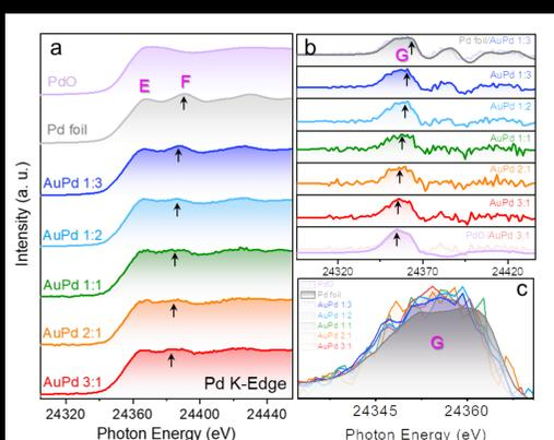
**Figure 3.** (a) Pd K-edges of AuPd nanoicosahedra along with Pd foil (bulk) and PdO for references. (b) Stacked and (c) overlaid first-differential spectra converted from (a).
