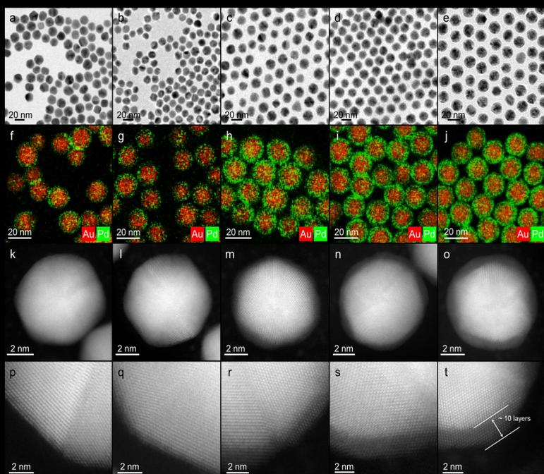
**Figure 1.** (a-e) Bright-field TEM images of core-shell AuPd nanoicosahedra made in different  $HAuCl_4/H_2PdCl_4$  ratios of (a) 3/1, (b) 2/1, (c) 1/1, (d) 1/2, (e) 1/3, and (f-j) their corresponding distributions of Au and Pd in the structures obtained by STEM-EDS mapping. (k-o) HAADF-STEM images of single AuPd nanoicosahedra taken from the samples in (a-e), and (p-t) atom-resolved HAADF-STEM imaging on one of their corner sites.
