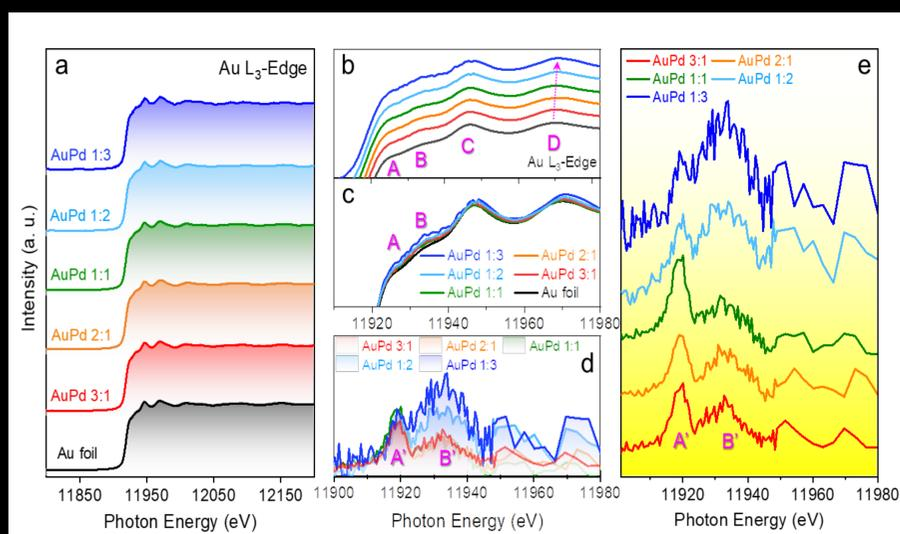
**Figure 4.** (a) Au  $L_{3}$ -edge of AuPd nanoicosahedra along with Au foil (bulk) for reference. (b) Stacked and (c) overlaid edge spectra in the interested energy range. (d) Derivative spectra obtained by subtracting the spectrum of Au foil from those of AuPd nanoicosahedra. (e) Evolutions in the features A' and B' revealed in the stacked spectra from (d).
