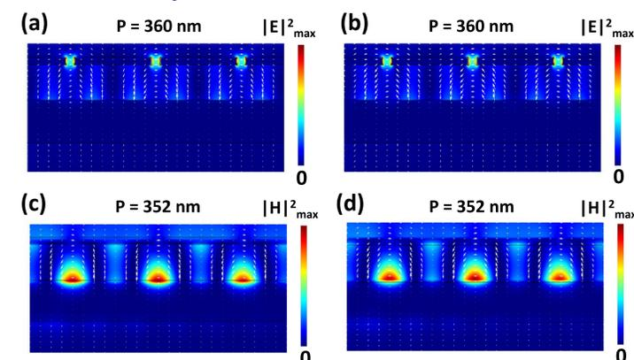
Figure 2 Electric field intensity ( $|E|^2$ ) and electric field ( $E_x + E_y$ ) distribution of the MIM-PDG structure at grating mode (a) before and (b) after H<sub>2</sub> adsorption.  $|E|^2$  and  $E_x + E_y$  at MIM mode (c) before and (d) after H<sub>2</sub> adsorption. The direction of the electric field has also been shown with arrows.
