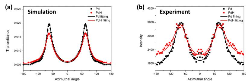
Figure 3 (a) Simulation of transmission intensity profile (dot) at different azimuthal angles before and after adsorption of 4% H<sub>2</sub>. (b) Transmission intensity profile (dot) on MIM-PDG before and after H<sub>2</sub> adsorption. The transmission profile is fitted (solid line) by using the Fano resonance model.
