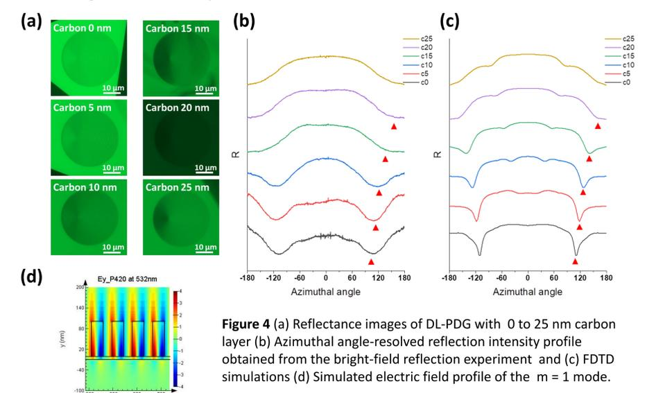
Figure 4 (a) Reflectance images of DL-PDG with 0 to 25 nm carbon layer (b) Azimuthal angle-resolved reflection intensity profile obtained from the bright-field reflection experiment and (c) FDTD simulations (d) Simulated electric field profile of the  $m = 1$  mode.
