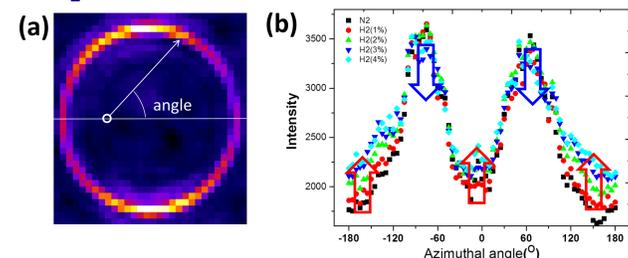
Figure 1 (a) Transmission intensity distribution after adsorption of 4% H<sub>2</sub> (b) Azimuthal angle-dependent transmission intensity profile after adsorption of H<sub>2</sub> from 0% to 4%.
