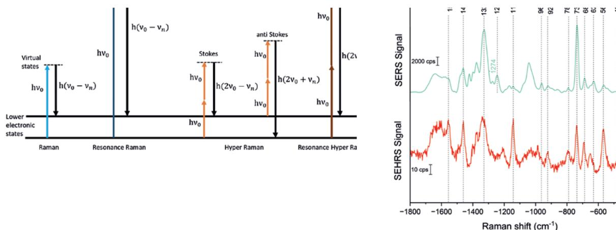
Fig. 1: Schematic representation of different vibrational scattering mechanisms
