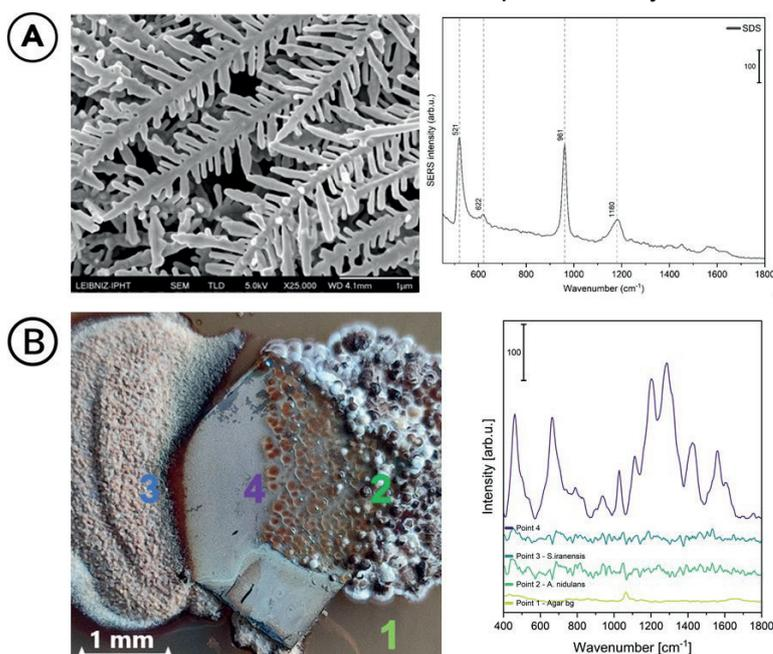
Figure 1 (A) SEM image of the SDS on the left and its spectrum on the right. (B) Spectra of *A. nidulans* and *S. iranensis* agar co-culture with SDS.
