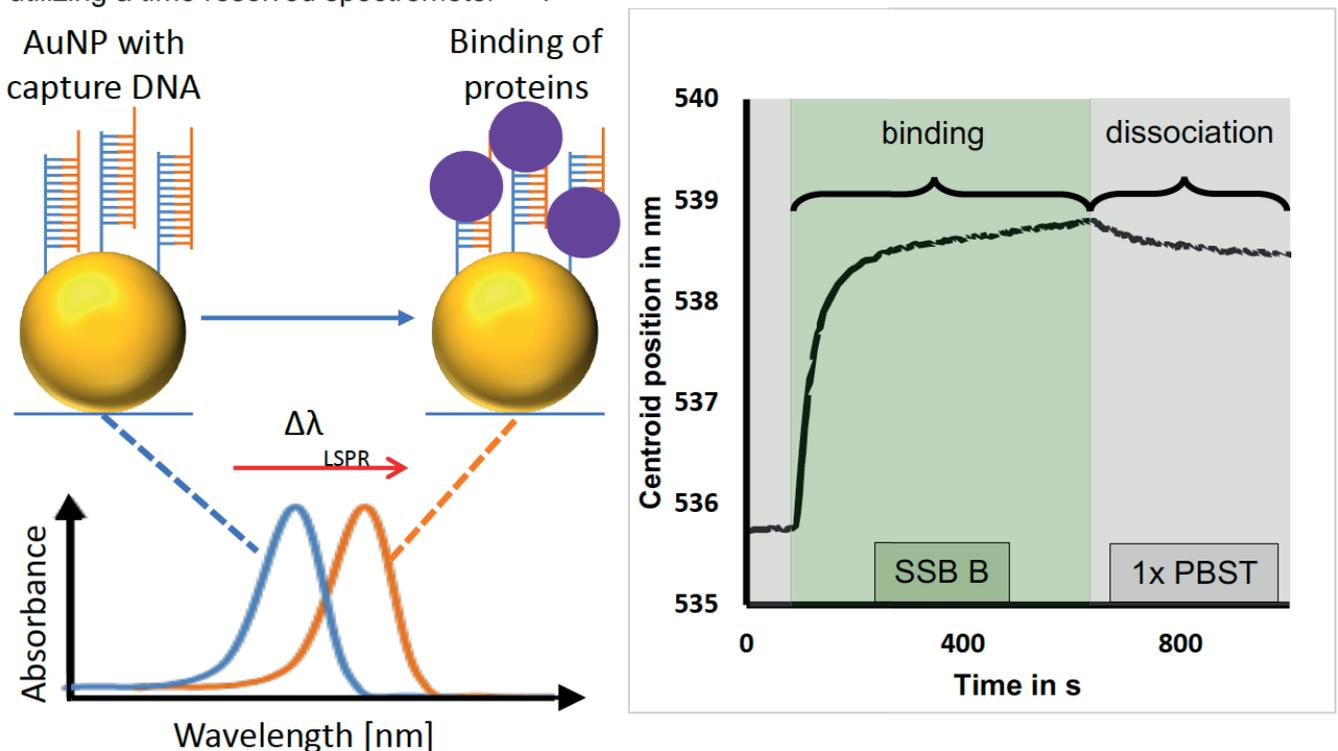
**Fig. 1: LSPR-based detection of DNA binding proteins interacting with DNA.**
