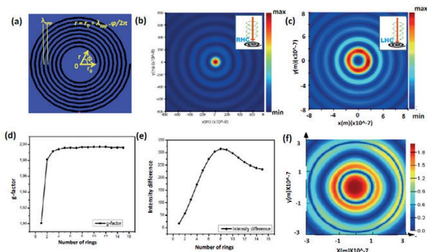
Fig. 1: Figure 1(a) The design of 8-ring LH-AS on a quartz substrate and its mathematical formulation in polar coordinate. (b,c) FDTD simulation results of 8-ring LH-AS with a bright and dark spot at the center, when excited with RH-CPL and LH-CPL (as shown in the inset). (d,e) the plot of  $g$ -factor and Intensity difference respectively with respect to the number of rings of AS. (f)  $g$ -factor map of the 8 rings AS with the maximum  $g$ -factor of 1.99 at the center.
