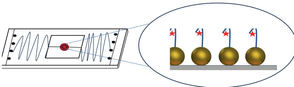
Fig. 1: Schematic representation of aptamer-gold nanoparticles on microfluidic chip.
