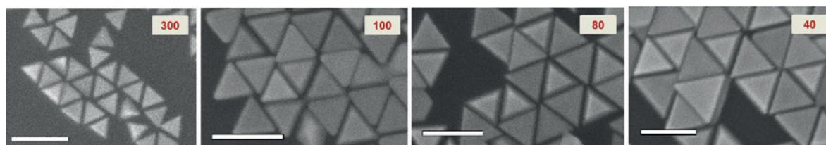
Fig. 1: Scanning electron microscopy (SEM) images of gold nanotriangles. Labels refer to the volume of intermediate seeds used in each synthesis. Scale bars are 100 nm
