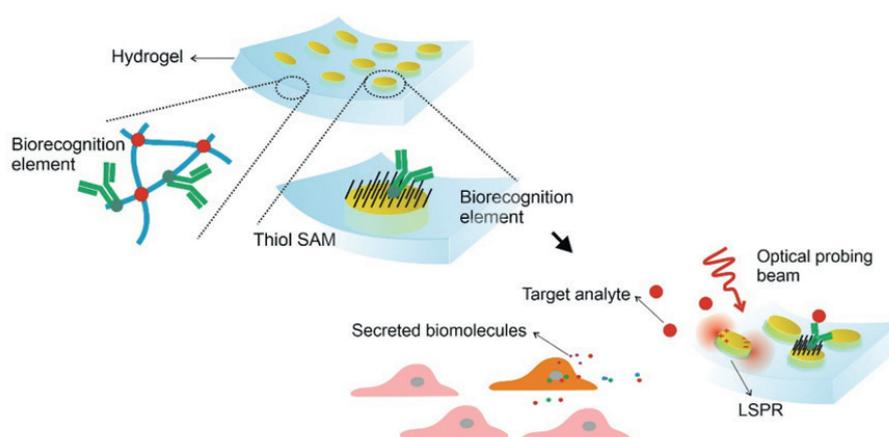
Fig.1: Schematics hydrogel element with biofunctionalized metallic nanostructures for a miniature sensing element detecting cellular-secreted species.
