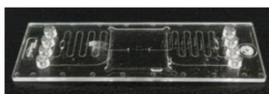
Fig. 2: Microfluidic chip applied in SERS experiments
