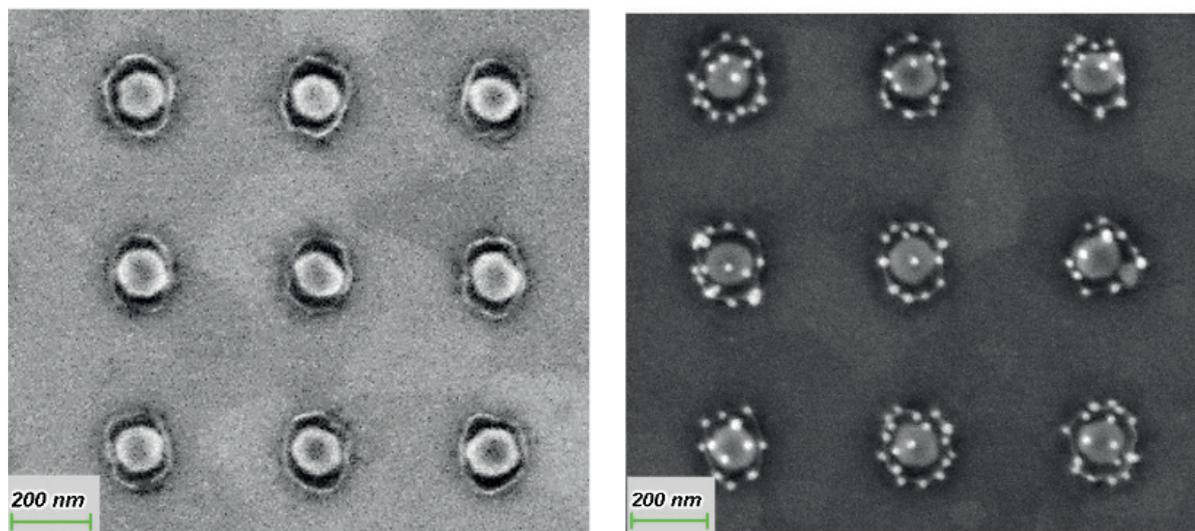
Figure 1: (a) SEM image of a square array of gold nanostructures (NSs) deposited on an indium tin oxide (ITO) substrate, after a plasmon-induced grafting of aryl film derived from 4-(aminomethyl)-benzene-diazonium-tetrafluoroborate; SEM image of a square array of gold NSs, after anchoring negatively charged gold colloidal particles on the NSs.
