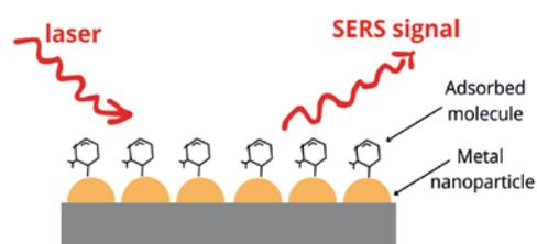
Fig. 3: Schematic illustration of the SERS detection
