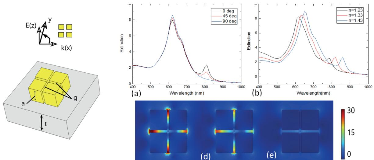
Fig. 1. The side view of gold nanocube quadromer cluster on  $\text{SiO}_2$  substrate. Nanocubes sides are 40 nm, and the gap  $g=5\text{nm}$
