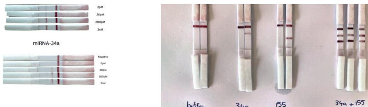
Fig. 1: Example LFA strips for the detection of individual miRNAs.
